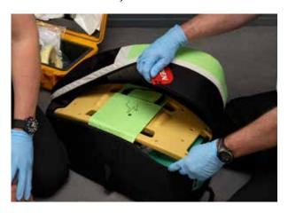
While the device is still in the bag, push the ON/OFF button for one second to power on the device. You will hear a few tones while the device does its self-test to make sure it's ready to operate before applying to the patient. There is a graphic on the green strap to remind the user to power ON the device while still in the bag.
