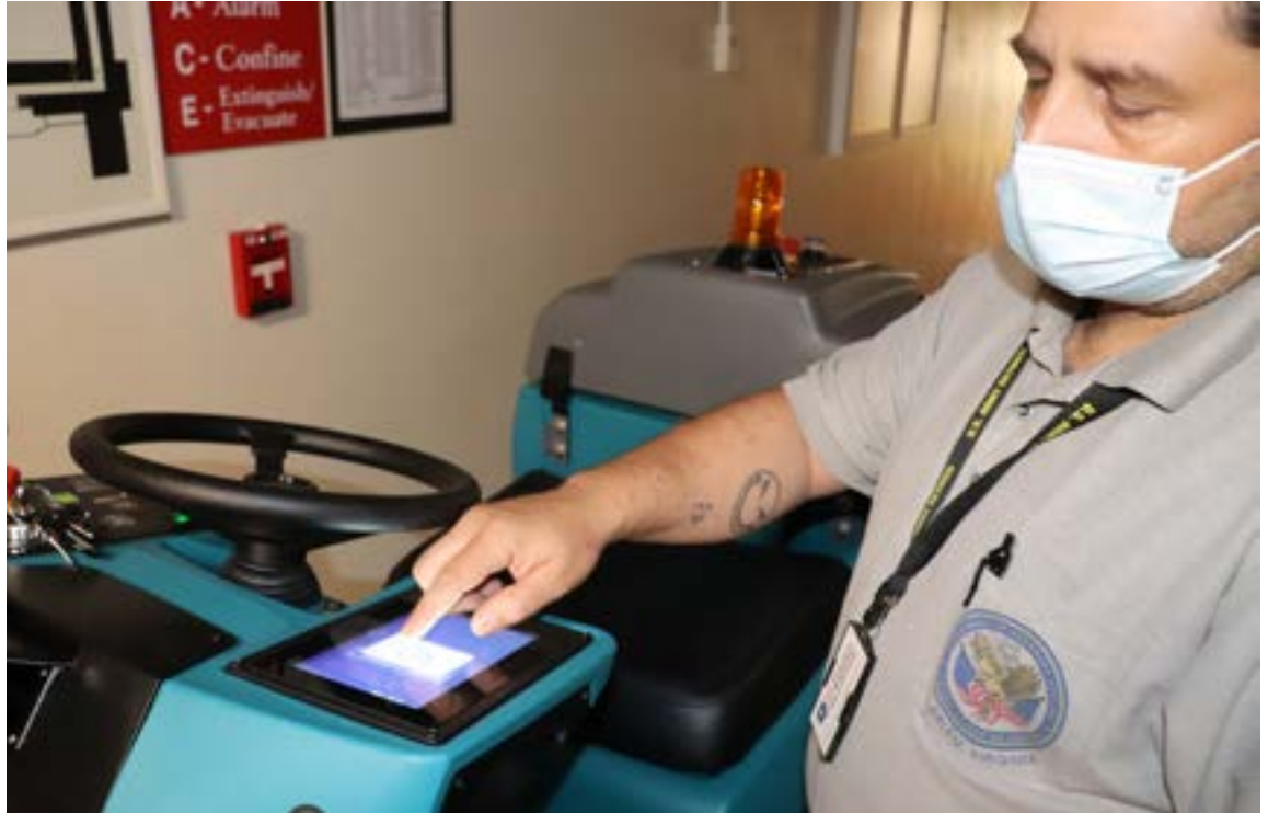
Jorge Markin, Third Shift Team Lead, sets the map option for a T380 AMR Autonomous floor scrubbing machine in Bldg. 74. The machines operate independently cleaning more than 10,000 square feet an hour, and free EMS staff to maximize high-value tasks such as keeping high-touch areas disinfected.
