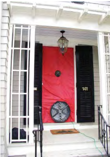
Fig. 6. (left) A blower door is used to depressurize a building by exhausting air at a rate that allows pressure gages and tracer smoke to measure the amount and location of air leakage. Photo: Robert Cagnetta, Heritage Restoration, Inc.
