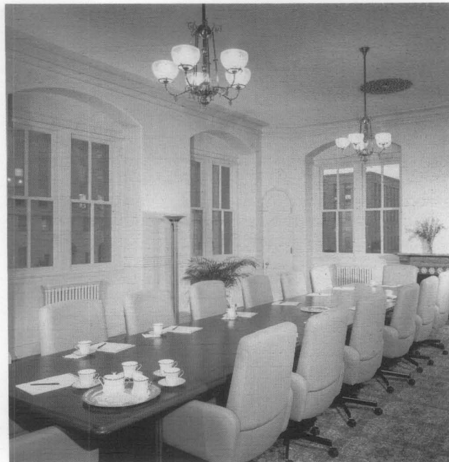
c. Conference room, Auditors Building, Washington, D.C. The historic steam radiators were retained for heating. The cast iron ceiling register was retained as a decorative element, but made inoperable to meet fire codes. Photo: Kenneth Wyner Photography courtesy of Notter Finegold + Alexander Inc.
