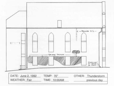
Fig. 13. Using sketch plans and elevation drawings to record the moisture damage along with the date, time, and weather conditions will show how moisture is affecting buildings over time. Drawing: Courtesy, Quinn Evans Architects.
