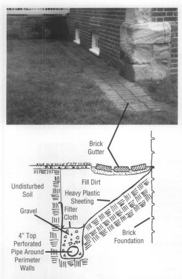
Fig. 18. This detail drawing shows a sub-surface perimeter drain in conjunction with a historic brick ground gutter system to help control roof run-off moisture from entering the historic foundation. Detail: Courtesy, Gunston Hall Plantation. Photo: Elizabeth Sasser.
