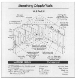
6. Often simple approaches, such as nailing plywood stiffeners between crawlspace studs and onto floor joist above and bolting sill plates to foundations can make a dramatic difference in protecting a building from seismic damage. Illustration: Reproduced with permission from Home Earthquake Preparedness Guide. EQE Incorporated, San Francisco, CA.
