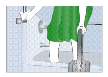
Install <u>safety rails</u> in the tub and shower. A <u>tub rail</u> fits tightly over the tub edge. Install <u>grab bars</u> at the front and side walls of the shower. Grab bars MUST be screwed into wall studs.
