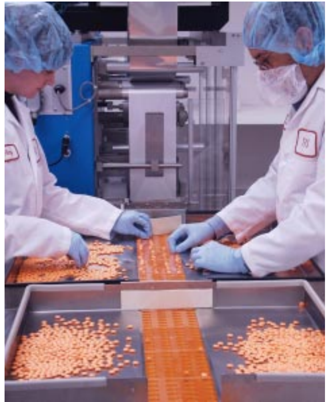
Amy Nicholson and Michael Chavez, both production controllers at the Clinical Research Pharmacy Coordinating Center in Albuquerque, N.M., flood fill blister cards.
