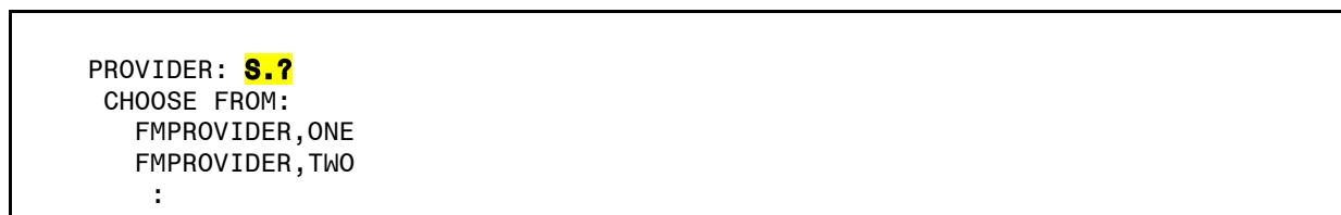
Figure 82: Field Types—Using the PREFIX and a Question Mark to Get a List of Entries in a Pointed-To File
